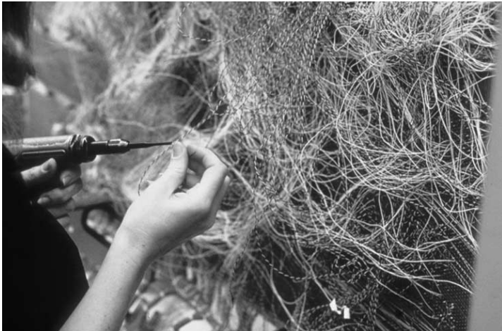
Figure 3. The 1110 was also the last system with a wire-wrap backpanel.
