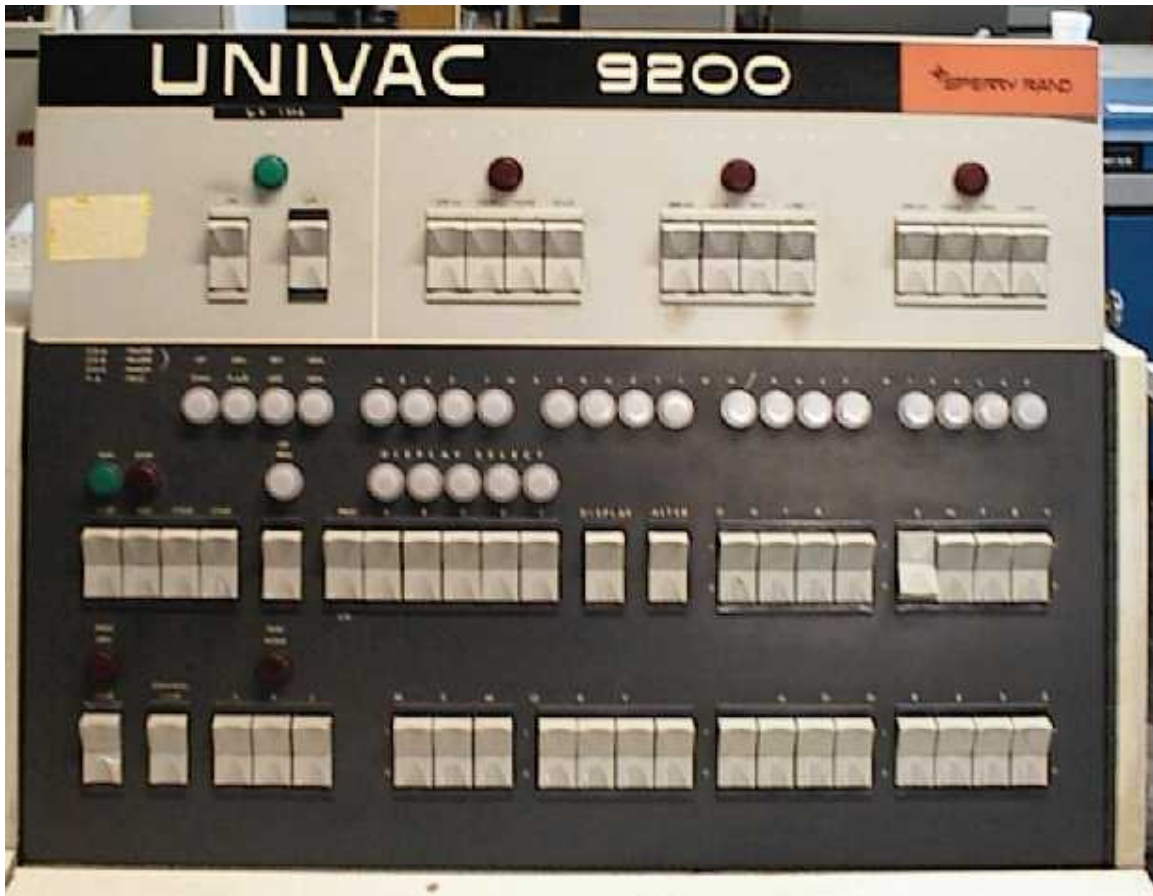
Figure 7: Console from a Univac 9200 Computer System
