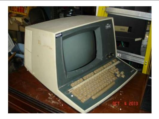
This terminal appears to have been manufactured in the middle 1970's as part of a stand-alone single-user word processing system, the Wang System 5. The terminal itself contains very little logic, beyond a parallel keyboard encoder. Video input is standard composite video fed into the terminal via a BNC connector on the rear bulkhead. Text output is via a parallel "Centronics" type connection. This is similar to the modular construction used on the Wang 2200 mini-computer.
