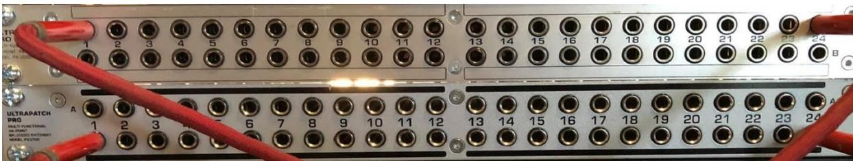
In the "Normalized" condition, the circuit connected (at the rear) to the top jack is automatically patched to the circuit connected (at the rear) to the bottom jack. In this way, the "Normal" state of connectivity is achieved without using any patch cords. By plugging in a patch cord to the "A" (top) jack, you can divert that signal to another location or device, using a simple patch cable. By plugging in a patch cord to
