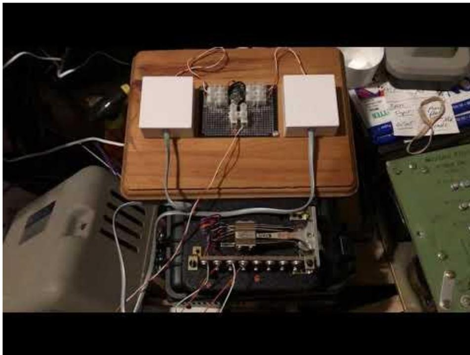
*Figure 5-Simple Common-Battery Telephone Circuit
