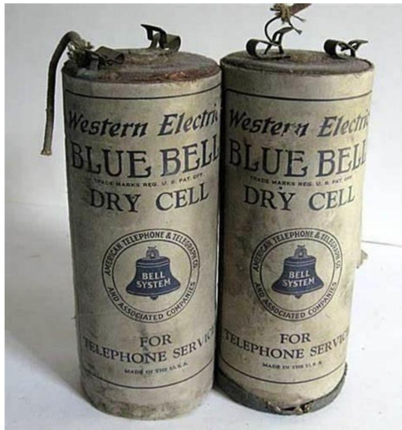
Figure 1-Dry Cell Batteries for Telephone Use
