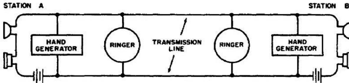
*Figure 4 - A Basic Point-to-Point Telephone Circuit*
