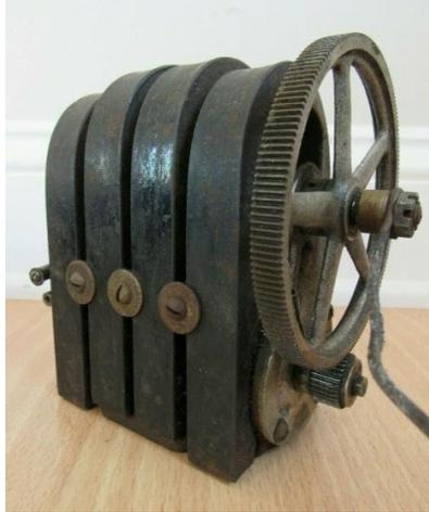
*Figure 2- A Four-Bar Magneto for Generating Ring Current*
